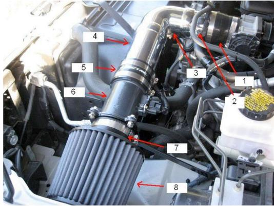
1. 3" ID to 2.75" ID hose adapter connected to throttle body with two hose clamps.
