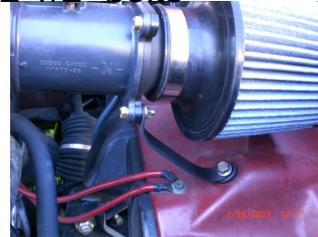
8. Spectre intake duct mounting plate connected to MAF tube with slight modification of holes.
