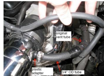
4. Spectre 90 Degree 3" elbow connected to vacuum adapter
